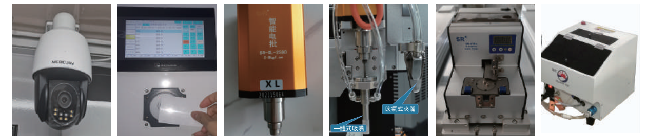
360度攝像錄影手機遠程監控 360-degree camera recording and mobile remote monitoring 設備密碼管控: 工卡 (IC卡) 刷卡登錄 Device password control: worker card (IC card) swipe card login 伺服智能電批 servo intelligent batc 視覺定位鎖附 Visual positioning lock with screws 吸附式供料器 Adsorption feeder 吹氣式供料器 Blowing feeder
