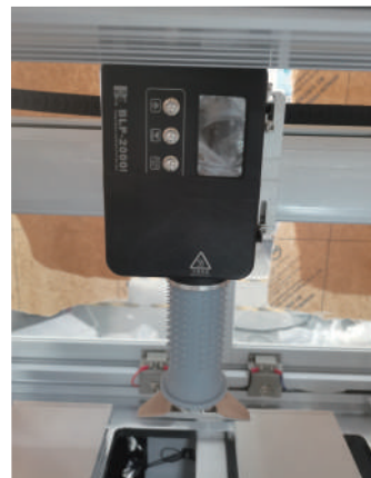
熱縮管加熱 Heat shrink tube heating
