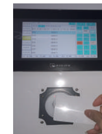
設備密碼管控: 工卡 (IC卡) 刷卡登錄 Device password control: worker card (IC card) swipe card login
